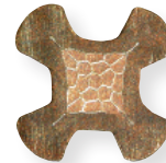
Indenter Crimp Cross-Section Across Axis
