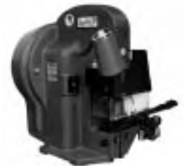
AMP-O-ELECTRIC Bench Machine with Special Applicator
