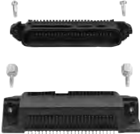
Screw Lock Hardware Kit Part Number 552631-1 Rear Panel Mount Only (One kit required per assembly) For pc board-to-panel applications (Panel thickness .062 [1.57] max.)
