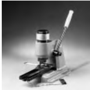
Bench press tooling Part Number 733280-3. This complete tool includes a Micro-MaTch dedicated tool set mounted on the bench press Part Number 654173-2.
