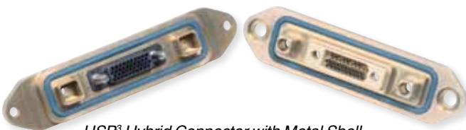
HSB 3 Hybrid Connector with Metal Shell and RF Contacts supplied by SV Microwave*
