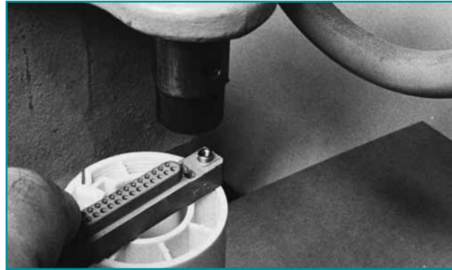
LOCKING/MOUNTING BUSHING ACCESSORY INSERTED INTO MB CONNECTOR BODY
