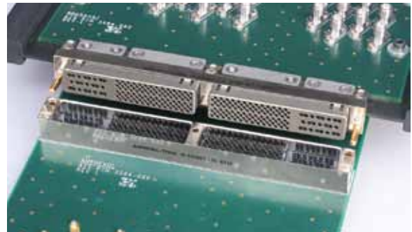
Hybrid Connector that has GigaStak-LG™ and DigiStak™ Inserts, shown on Testing Boards
