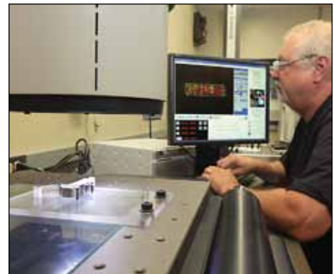
Checking for dimensional accuracy of LRM parts and heatsinks.
