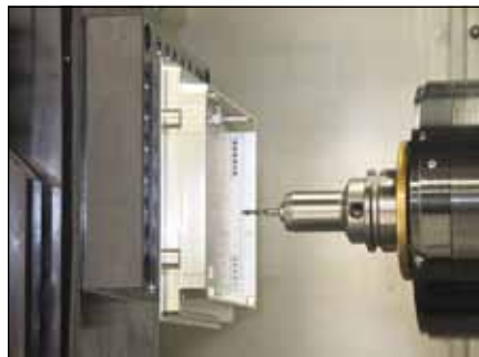
Close-up photo showing vertical machining of heatsink housings done at Amphenol.
