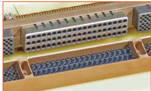
Module and backplane with LVDS differential pair brush contacts
