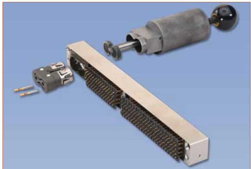
Exploded view - tool 10-507924-1 has removed power module from backplane. (size 22D contacts shown removed)
