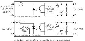
Random Turn-on Units have a Random Turn-on circuit instead of Zero Voltage Circuit
